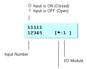
\* indicates that communication has been established with the I/O Module
