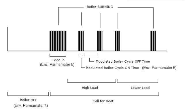
The OFF time is a function of the system loading and may be adjusted by a tweaking factor, environmental parameter 7.
