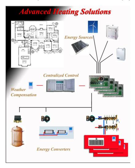
This document details programming and diagnostic features of the RadMaster® central console. The console is the central point of control. It communicates to all other components over local network and manages all system processing.
