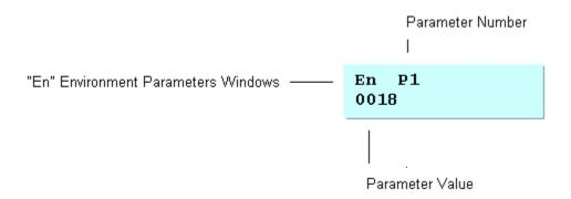
Press to change the system parameter number. Use Numerical keys to enter the parameter value.
