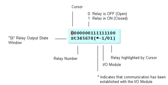
Press to change I/O Module. Press and to move the cursor. Press to activate or deactivate a relay.
