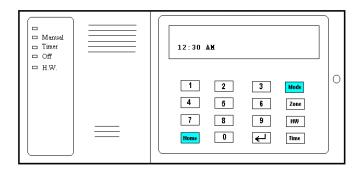
The MODE key changes the setup/diagnostic context (e.g. moving from Sensor Communication States to I/O module output statues).
