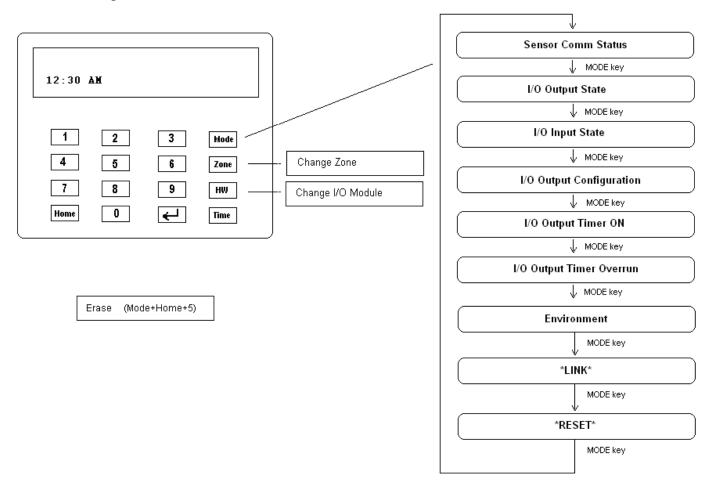
The HW key increments the module when viewing module related data (e.g. I/O Output State or I/O Input State etc).
