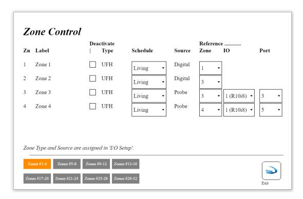
Zone Type and Source can only be changed from the "IO Setup" screen. They cannot be overridden.
